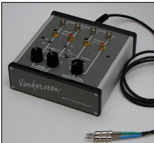
Photo 5: The Arta-2 measuring unit can be connected to a sound card.
