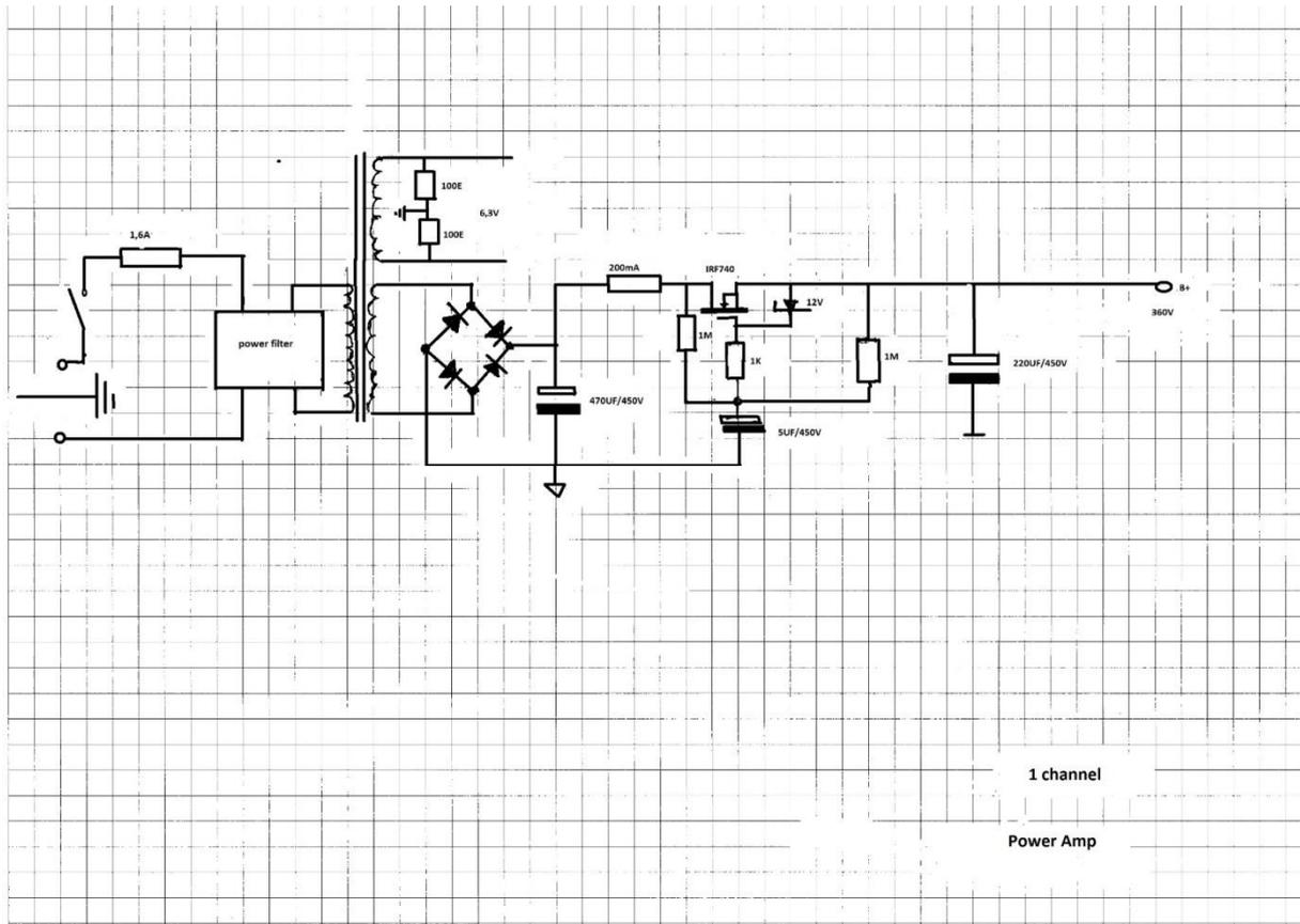
The power transformer is the VDV-POW80. The circuit around the IRF740 acts as a super capacitor, highly rejecting any hum on the B+ line. The ripple voltage on B+ = 360 V is smaller than 1 mVrms. This B+ circuit can drive both channels. Only 6,3 Vac is needed for to drive the filaments of the power tubes, grounded by two 100 Ohm resistors.
