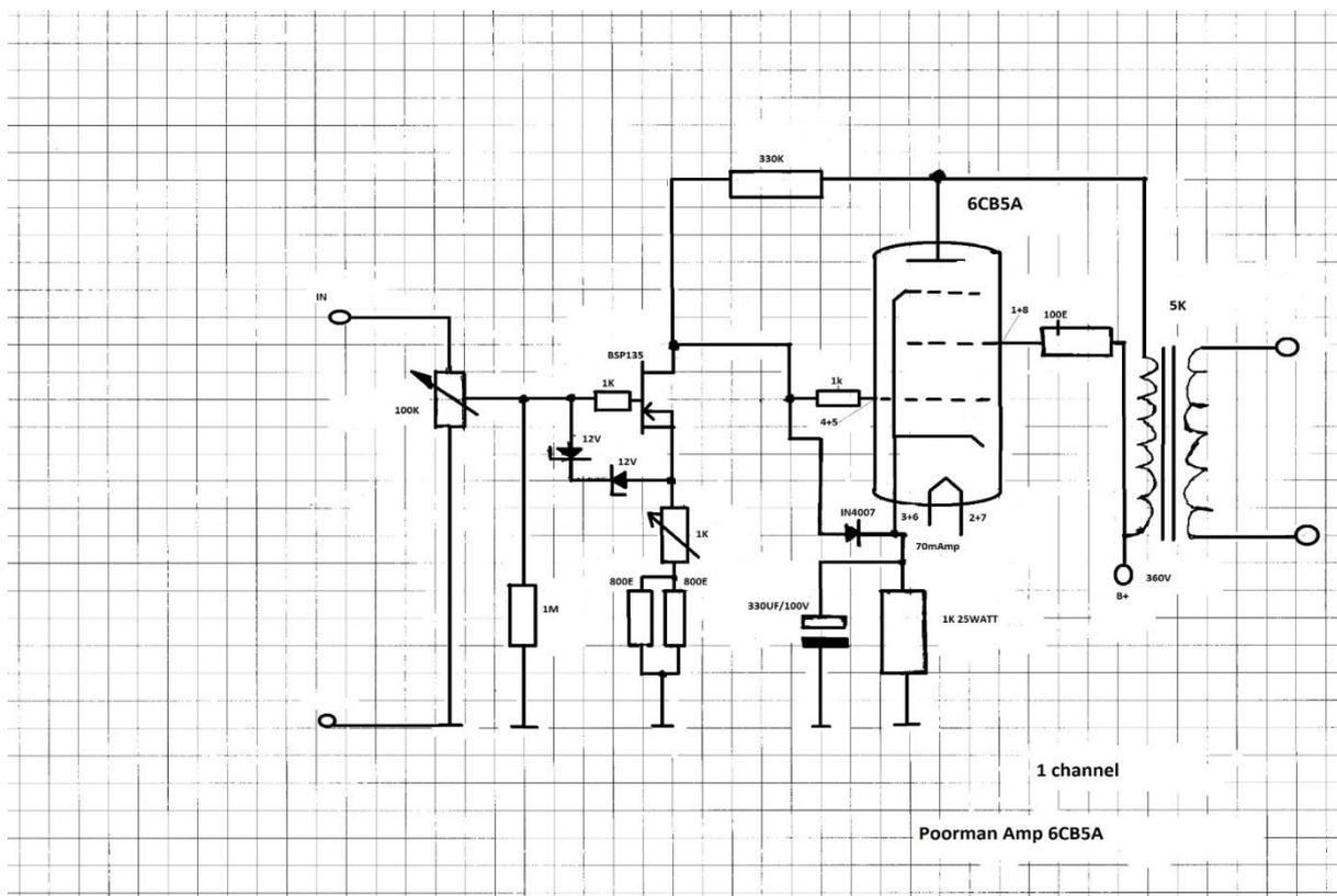
The BSP135 functions as a voltage controlled current source. The two 12 V zener diodes protect the FET at startup of the amplifier. The adjustable source resistor (1k) sets the quiescent current (70 mA) of the 6CB5A power tube (measure 70 V over the 6CB5A cathode resistor of 1 kOhm).
