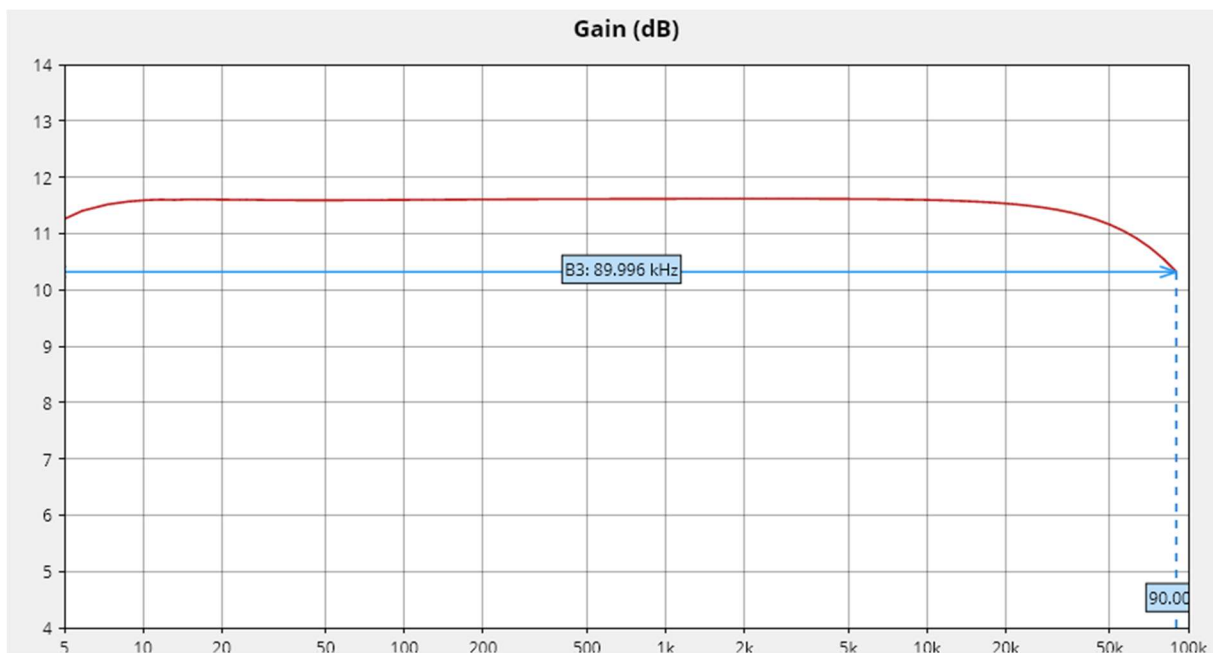
Figure 14 - Measured gain vs frequency
