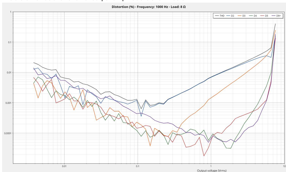
Figure 26 - Distortion vs output amplitude
