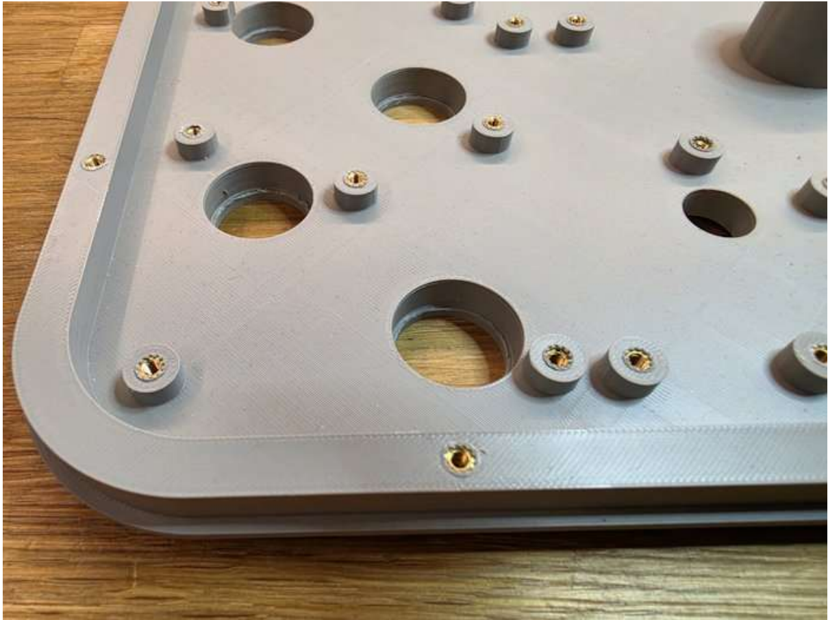
Figure 40 - M3 inserts are used. The topside of the enclosure is shown here upside down.
