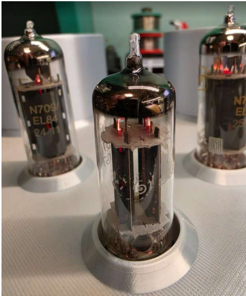
Figure 43 - All glowing well. The pla does not get soft at all.
