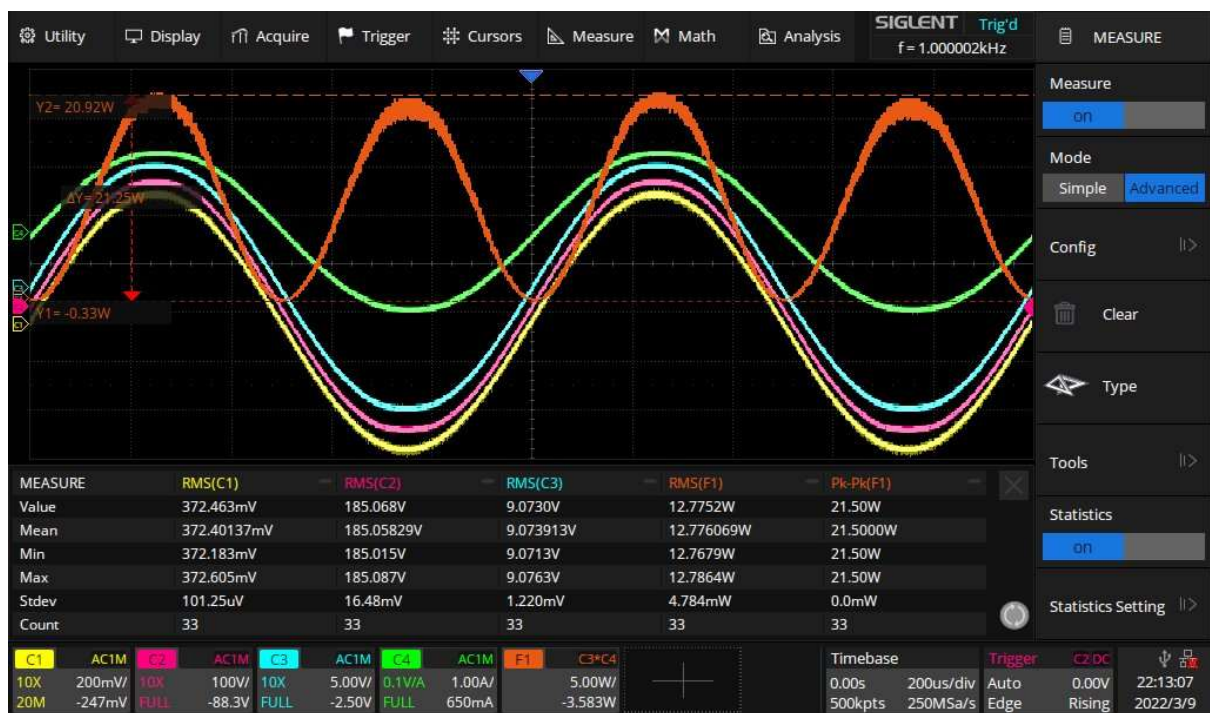
Figure 13 - Oscilloscope power measurement of the breadboard circuit
