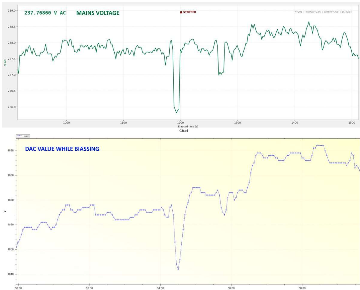
Figure 23 - Correlation between mains voltage and DAC value when biasing
