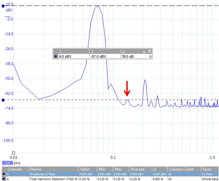
Fig. 6: AB test with 70 Hz signal +9 dBV (= 1 W in 8  $\Omega$ )
