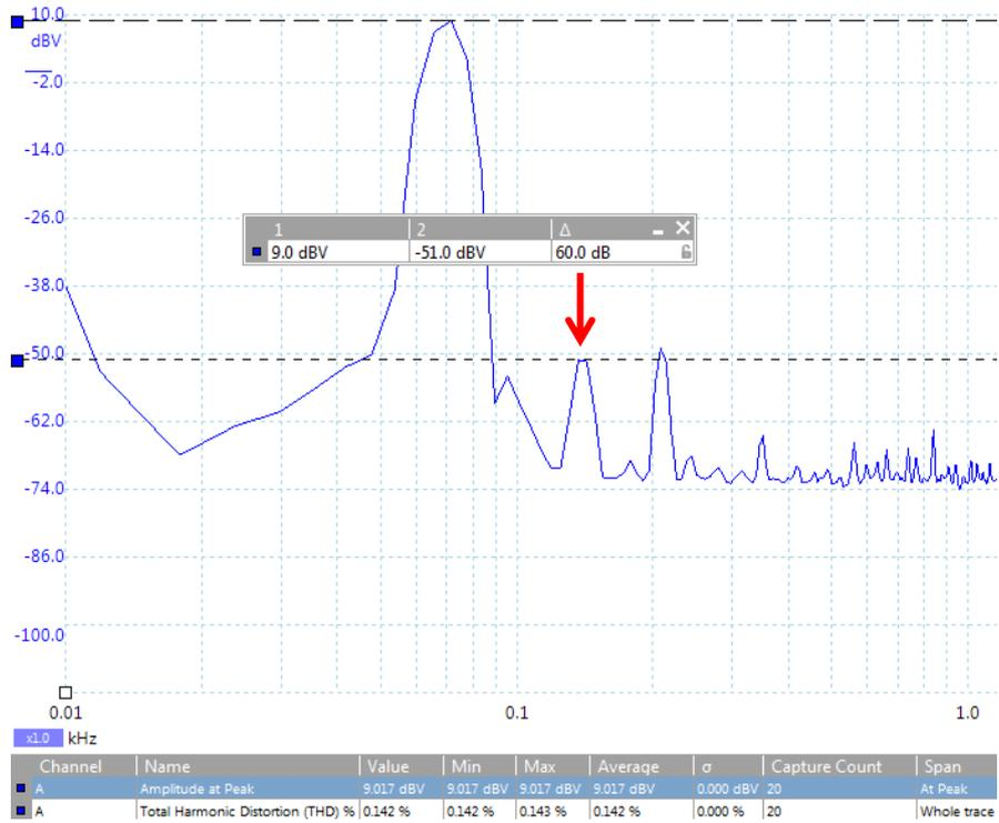
Fig. 5: AB test with 70 Hz test signal +9 dBV (= 1 W in 8  $\Omega$ )
