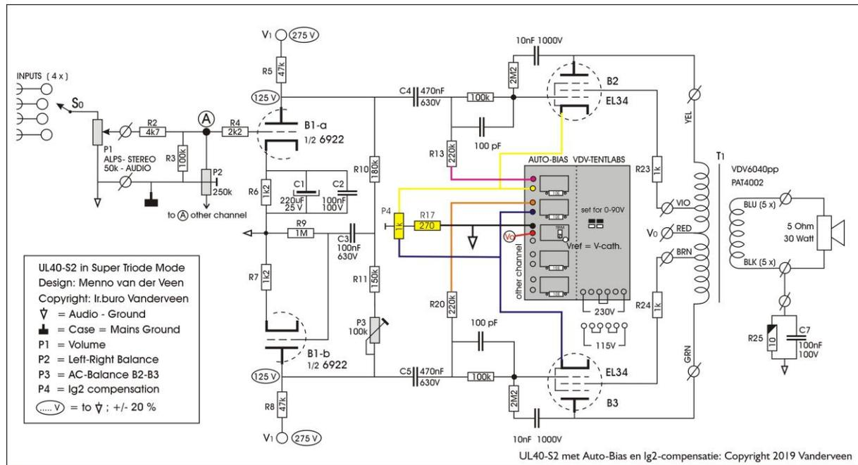
Fig. 1: UL40-S2 Auto-Bias circuit with  $I_{g2}$  compensation
