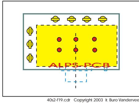
12. Mount on the Alps-PCB (smallest PCB) 7 solder terminals on the side with the wire-pattern. Align them according to figure 19 en solder them.
