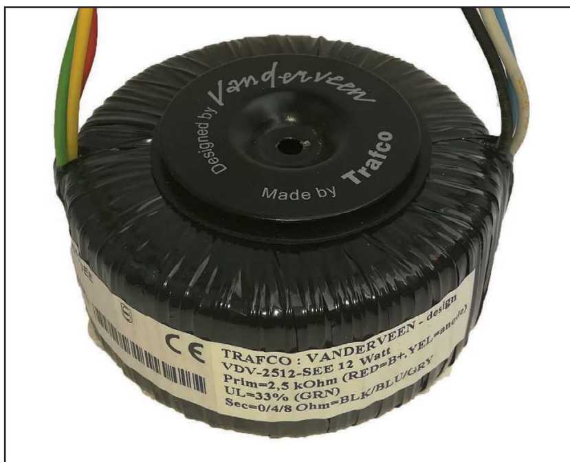
Figure 4: The Trafco-Vanderveen toroidal OPT as applied in the Trans-SE10 amplifier
